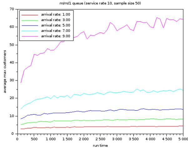
FIGURE 3.  $N_{max}$  as a Function of Runtime, as Obtained by Simulation.
