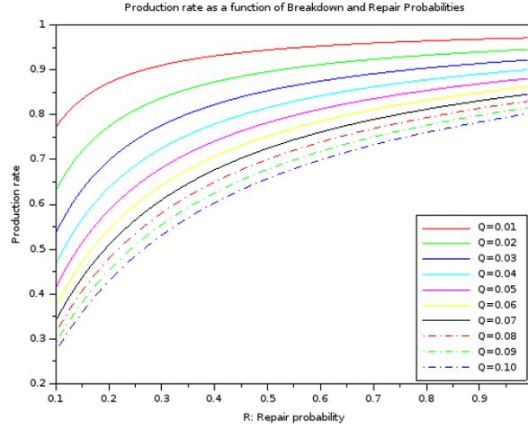
FIGURE 5. Production Rate as a Function of Breakdown and Repair Probabilities.
