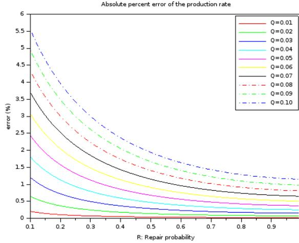
FIGURE 7. Absolute Percentage Errors as Functions of Model Parameters.
