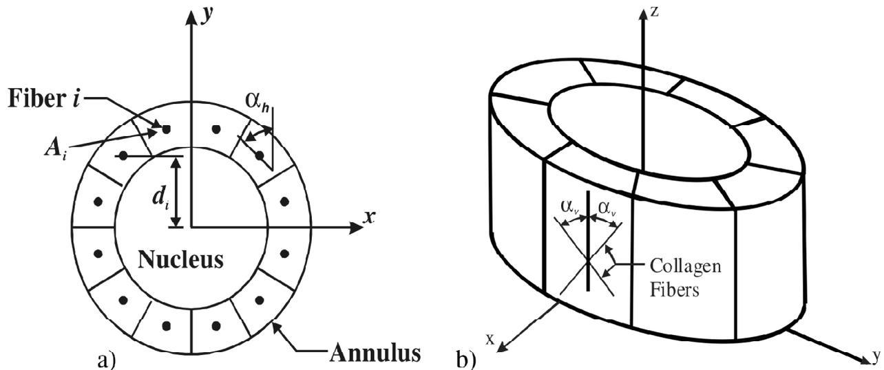
Figure 3: Intervertebral disc model: (a) basic cross-sectional geometry; (b) annulus collagen fiber orientation
