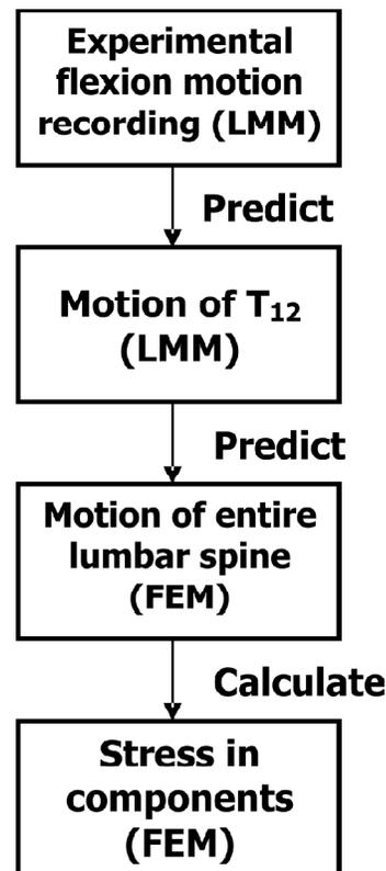
Figure 5: Flow chart for the overall solution procedure
