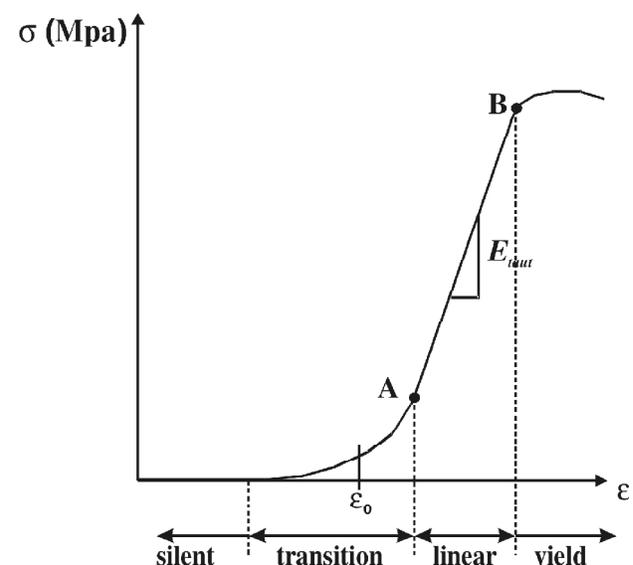
Figure 2: General shape of the ligament stress-strain curve (after Chazal *et al.*, 1985)
