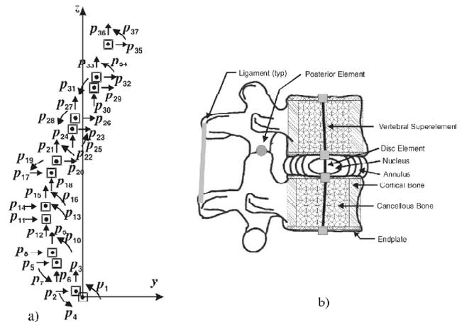
**Figure 1: Overall model geometry and components: (a) model nodes and degrees-of-freedom, (b) motion segment detail including all component elements**
