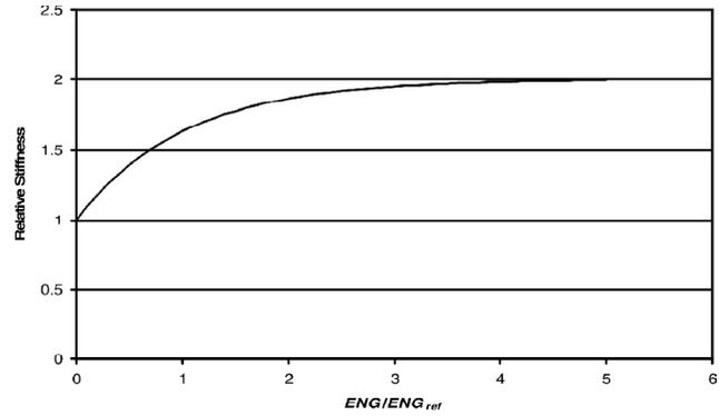
Figure 4: Variation of elastic modulus with component energy
