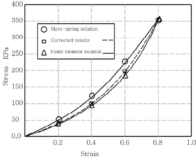
**Figure 2: (Right) the nonlinear FEM solution, (Left) the regular MSS solution for a 10%PVA rectangular pate (5 x 15 cm<sup>2</sup>) for a deformation starting form 15% to 100%**
