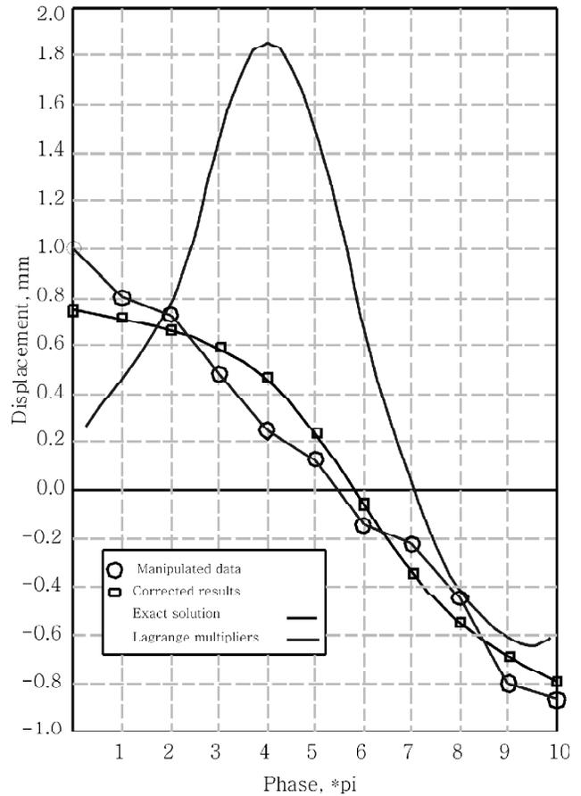
**Figure 3: Motion of the vibrating spring for  $k=1$ , manipulated and modified results**
