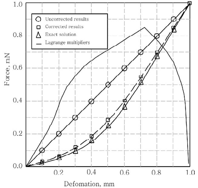
**Figure 1: Modeling of a parabolic spring with a linear spring in a MSS - the exact solution and modified results are in the same range with 10% difference**
