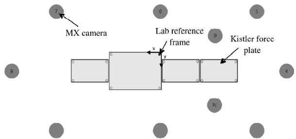
**Figure 3: Force Plates and Cameras Configurations**
