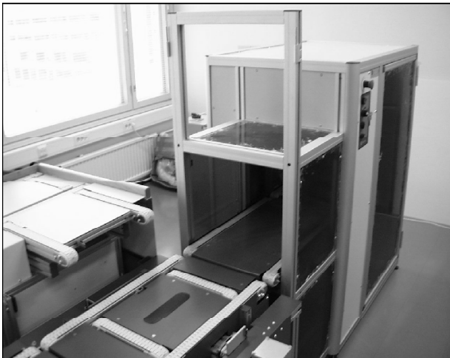
Figure 6: Lifter Installation in the Assembly Line
