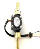
Fig 3.6 Arduino water flow sensor
