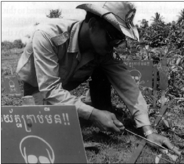
Figure 2: Mine Detection using Contact Probes
