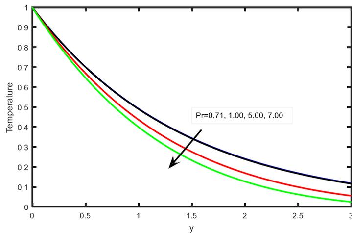
Fig.13. Temperature profiles for different values of Prandtl number (Pr).
