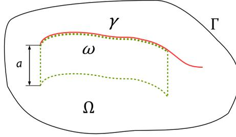
FIGURE 1. Geometry of the cracked body with a volume rigid inclusion.
