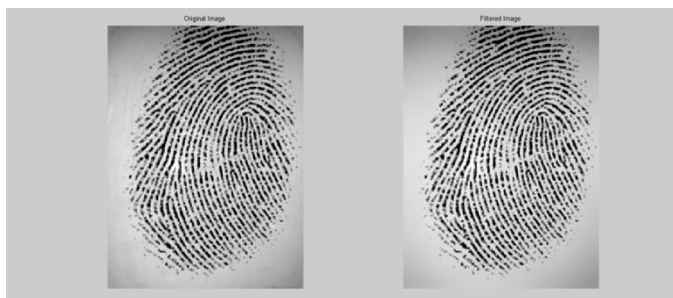
Fig 4: Fingerprint enhancement (a) original image (b) Enhanced image with integration constant= 0.1, gradient modulus threshold=5
