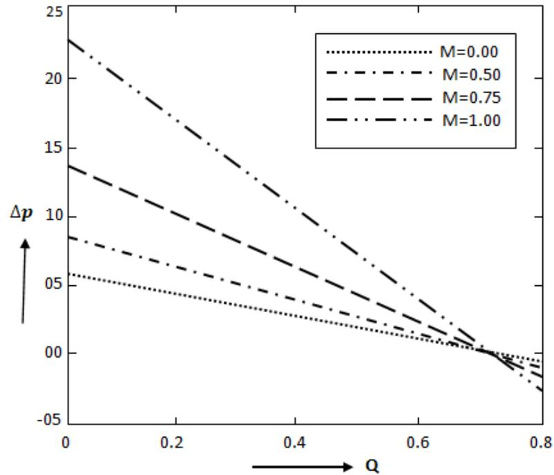
Fig. 3(a): Variation of the pressure rise with flow rate for different values of  $M$  when  $\alpha = 0.1$ ,  $\varphi = 0.4$
