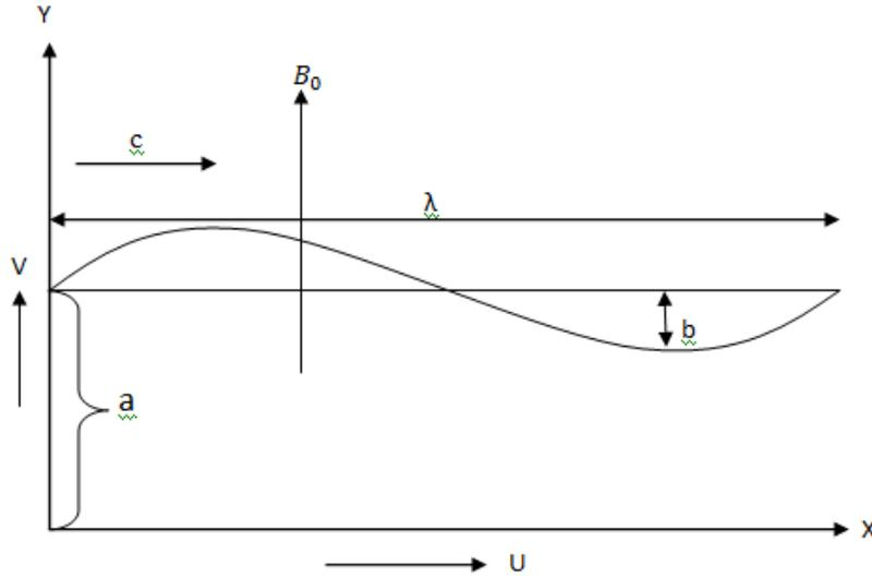
Fig 1. Geometry of the peristaltic flow
