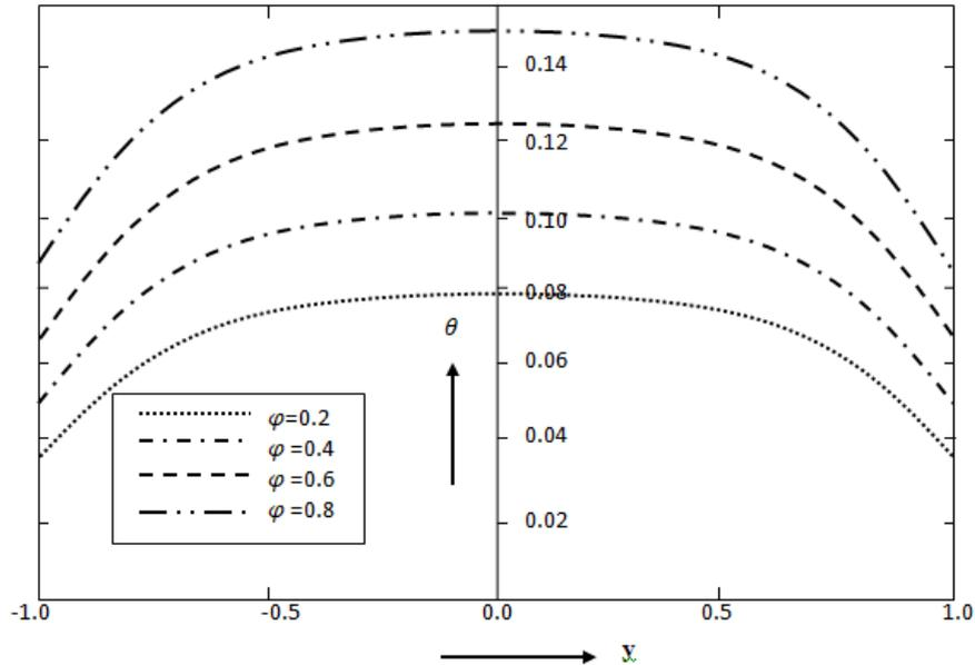
Fig. 5(c):Variation of temperature with  $y$  for different values of  $\phi$ , when  $\alpha = 0.1, Br = 0.3, Q = 0.3, M = 0.4, x = 0.4$
