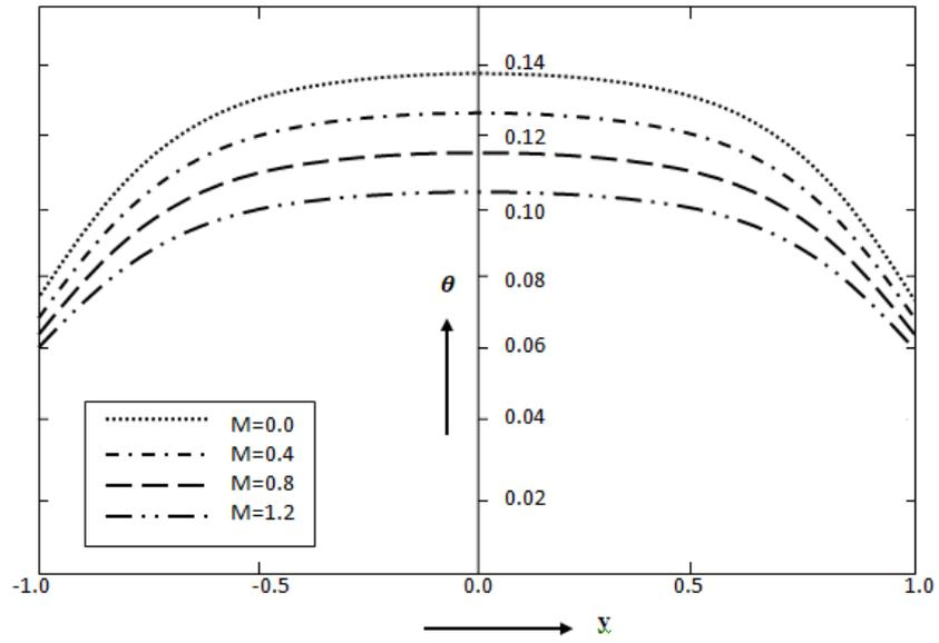
Fig. 5(a) Variation of temperature with  $y$  for different values of  $M$ , when  $\alpha = 0.1$ ,  $\varphi = 0.4$ ,  $Q = 0.3$ ,  $Br = 0.3$ ,  $x = 0.4$
