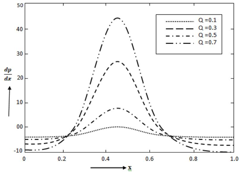
Fig. 2(b): Variation of the pressure gradient with  $x$  for different values of  $Q$  when  $\alpha = 0.1$ ,  $M = 0.4$ ,  $\varphi = 0.4$
