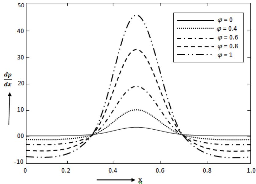
Fig. 2(d): Variation of the pressure gradient with  $x$  for different values of  $\varphi$  when  $Q = 0.3$ ,  $M = 0.4$ ,  $\alpha = 0.1$
