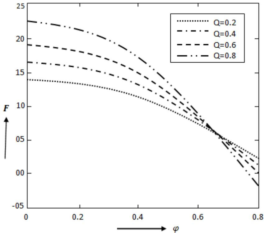
Fig. 4(b) Variation of the friction with amplitude ratio for different values of  $Q$  when  $\alpha = 0.1$ ,  $M = 0.5$
