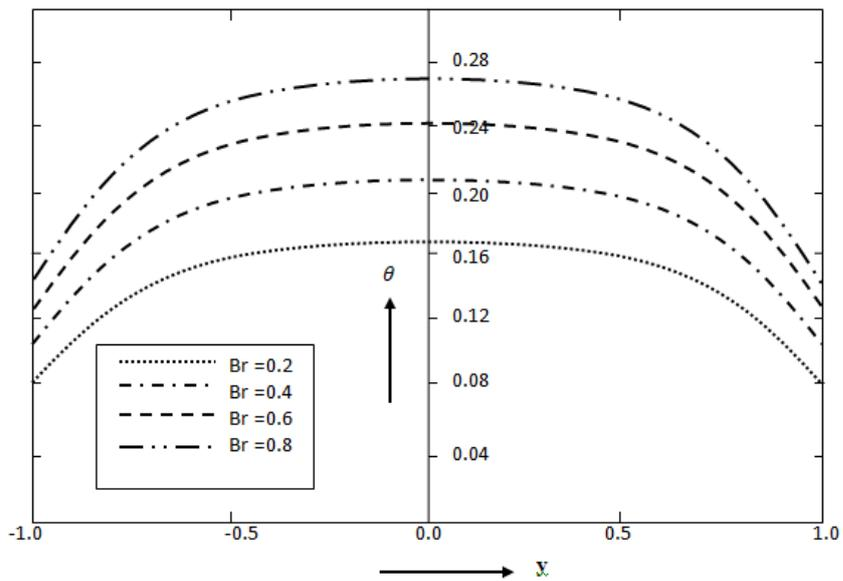
Fig. 5(b) Variation of temperature with  $y$  for different values of  $Br$ , when  $\alpha = 0.1$ ,  $\varphi = 0.4$ ,  $Q = 0.3$ ,  $M = 0.4$ ,  $x = 0.4$
