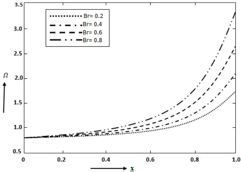
Fig. 6 (b): Effect of heat transfer coefficient with x for different values of Br, when  $\alpha = 0.1$ ,  $\varphi = 0.4$ ,  $Q = 0.3$ ,  $M = 0.5$ .
