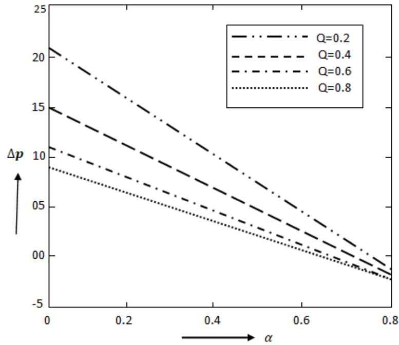
Fig. 3(c): Variation of the pressure rise with parameter of Pseudoplasticity( $\alpha$ ) for different values of  $Q$  when  $\phi = 0.4$ ,  $M = 0.5$ ,
