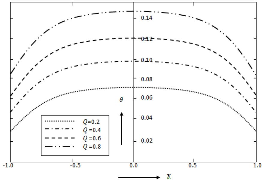
Fig. 5(d):Variation of temperature with  $y$  for different values of  $Q$ , when  $\alpha = 0.1, Br = 0.3, \phi = 0.4, M = 0.5, x = 0.4$
