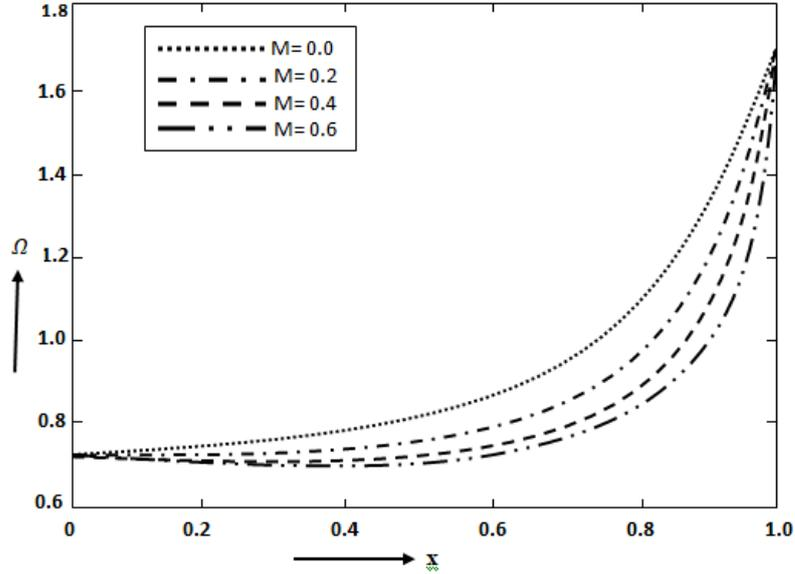
Fig. 6 (a): Effect of heat transfer coefficient with x for different values of M, when  $\alpha = 0.1$ ,  $\varphi = 0.4$ ,  $Q = 0.3$ ,  $Br = 0.4$ .
