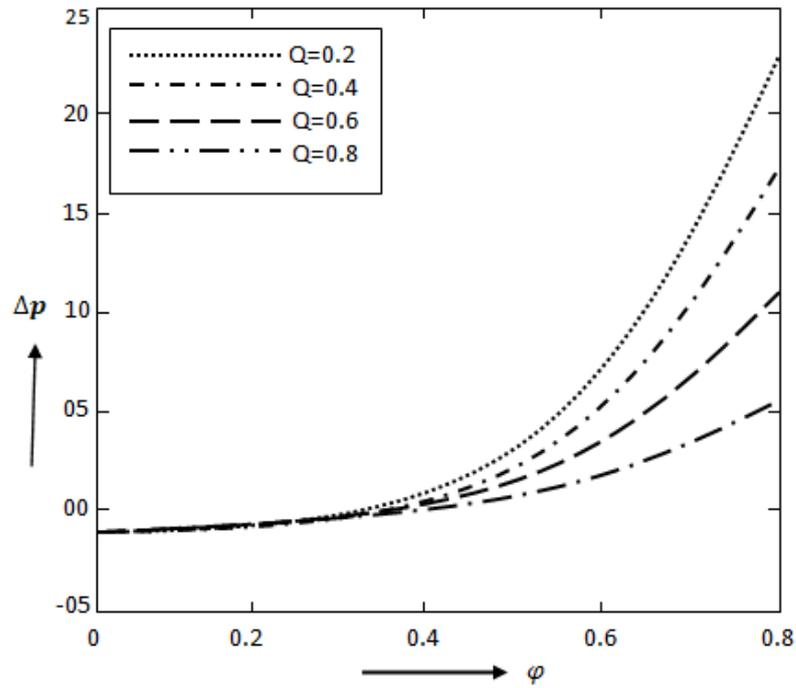
Fig. 3(b): Variation of the pressure rise with amplitude ratio for different values of  $Q$  when  $\alpha = 0.1$ ,  $M = 0.5$ ,
