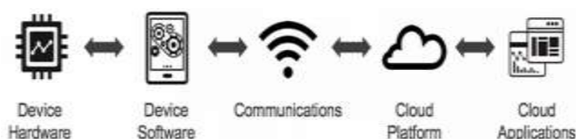
The IoT Technology Stack
