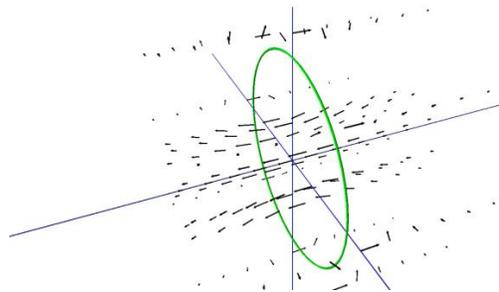
Fig. 1. Magnetic field of a circular coil.
