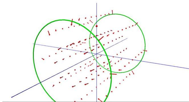
Fig 3. Magnetic field of a magnetic bottle. The red dot is the initial position of a charged particle
