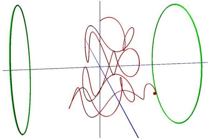
Fig. 4a Trajectory of a charged particle in a magnetic mirror
