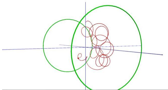
Fig. 4b Trajectory of a charged particle in a magnetic mirror, alternate view
