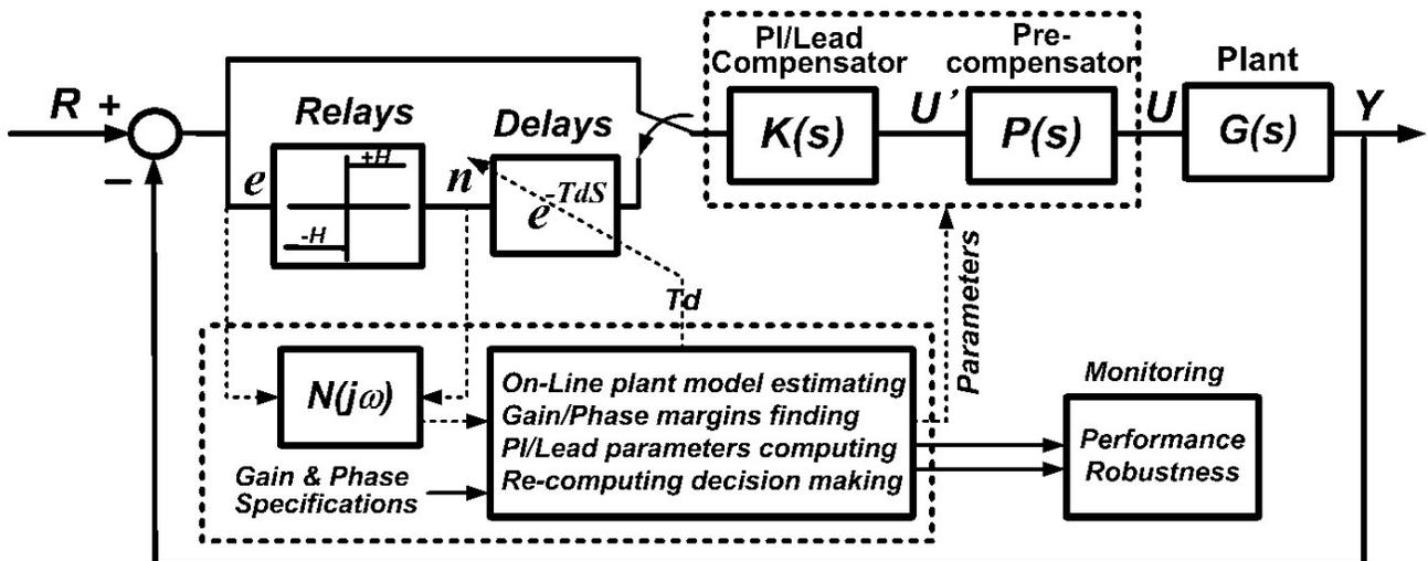
Fig. 1: The On-line Computing and Control Structure
