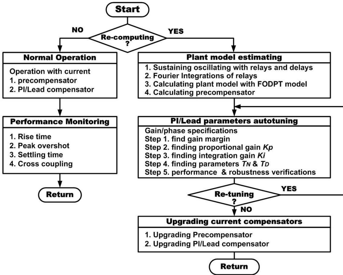
Fig. 2: The Flow-chart of the On-line Computing and Control
