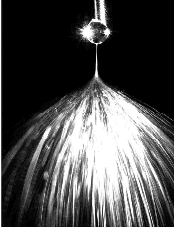
Figure 2: Photograph of Electrostatically Spun Fibres 14% Concentrated Polyvinyl Alcohol. This Image was taken with Nikon D70 Camera at a Shutter 250 ms Using a Nikkor Makro 60 Lens, Using Laboratory Needle Spinner and Rounded Disk as a Collector Fixed in a Distance 60mm From A Needle Tip, with Applied Voltage 14kv
