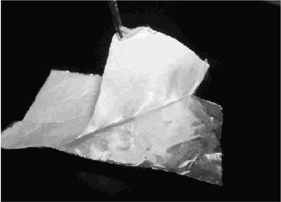
Figure 3: Non-woven Poly(L-lactide) Nanofibrous Web could be Easily Peeled off the Aluminum Foil
