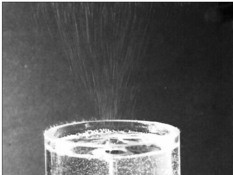
Figure 2: Multiple Jets Ejected from an Aerated Polymer Solution in a Electric Field
