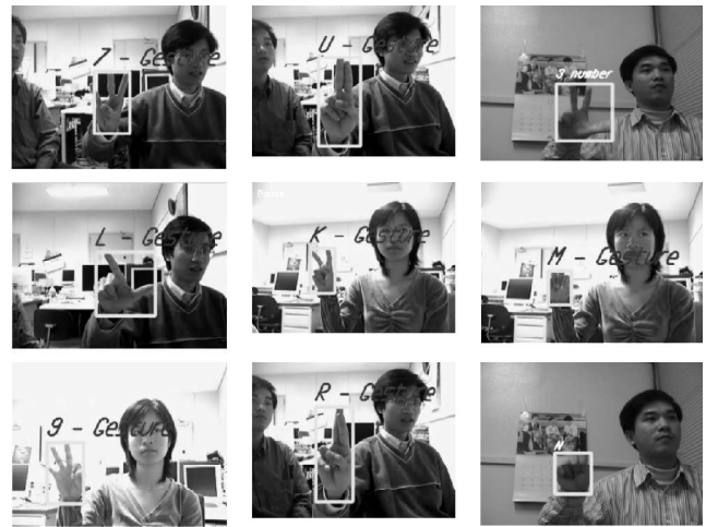
Figure 14: The results of the hand gestures recognition
