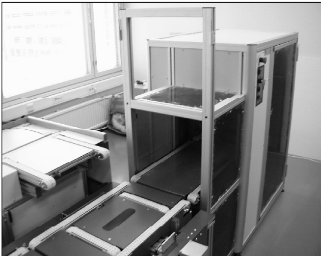
Figure 6: Lifter Installation in the Assembly Line
