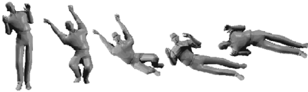
Figure 9: Zero angular momentum maneuvers illustrating a rotation in X axis
