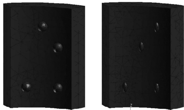
Figure 11: Discretization of lamella inclusion; spherical (left) and ellipsoidal (right)
