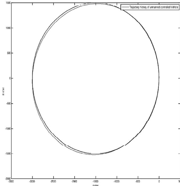
**Figure 8:** Predefined Trajectory (red-line) and Tracking Result (Black-line)
